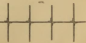
Bilge-keelsons, &c.—In putting on the lug-pieces for keelsons, see that they are quite fair with the edge of inside flange of angle-iron frame, and the fore-and-aft flange of reverse frame.
